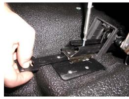
Slide guide brackets into seat rail and loosely attach #10 x 3/4" Phillips pan head machine screws
